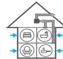
MEV units have a single extract fan with multiple connections to extract air from each 'wet' room in a home with a single exhaust to outside. The units are a little smaller than MVHR with fewer duct connections so may fit where MVHR doesn't.
