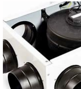
MEV units have a single extract fan with multiple connections to extract air from each 'wet' room in a home with a single exhaust to outside. The units are a little smaller than MVHR with fewer duct connections so may fit where MVHR doesn't.
